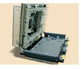
**Finished Board Test Fixtures** require dimensional stability and high mechanical strength to ensure accurate readings.
